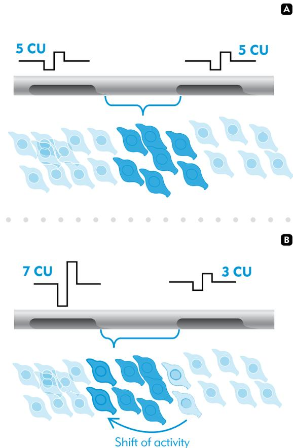
**Figure 1.** Diagram of active current steering whereby in the first example (A), half the current (CU—clinical units) is “steered” to each of two neighboring electrodes so that the locus of stimulation is approximately halfway between the two contacts. In the second example (B), as a greater proportion of current is steered toward one of the electrodes, the locus of stimulation is shifted closer to that electrode.
