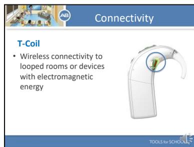
Finally, let's talk about the Naida's T-Coil. It is built into the Naida and allows for wireless connectivity to looped rooms or devices with electromagnetic energy. The T-Coil is enabled through a program setting by the child's audiologist. You will need to check with the child's parents or audiologist to determine if a T-Coil program is available.
