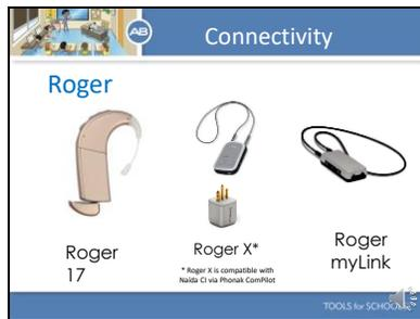
An FM or Roger system is commonly used in many classrooms. It is a wireless system that transmits the teacher's voice directly to a student's cochlear implant or hearing aid. It significantly improves the signal to noise ratio in difficult listening environments by overcoming noise and distance. The student wears the receiver and the teacher wear the microphone.
