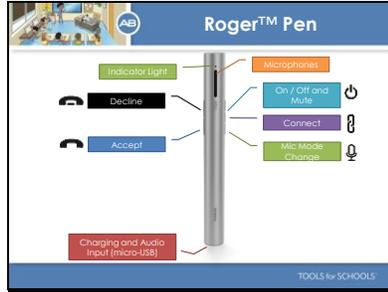
Here is the Roger Pen. It is a small versatile microphone that can be used for various listening situations. It also features Bluetooth® connectivity so it can be used with the phone and any device that has Bluetooth capabilities. It is great for older children and teenagers as it allows for personal management of Roger.
