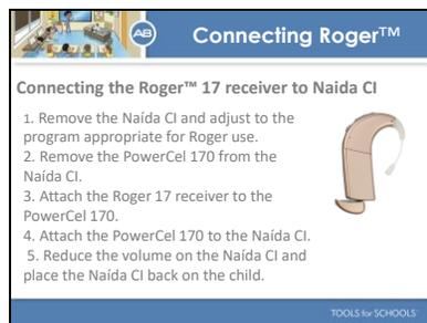
The steps for connecting the Roger 17 to the Naida CI are listed over the next 2 slides. Begin by removing the Naida from the child and adjusting the processor to the appropriate program for Roger use. Next remove the battery. Attach the Roger 17 to the battery and then reattach the battery to the Naida. Reduce the volume and place the processor back on the student. Keep in mind most older children are able to manage these steps on their own.
