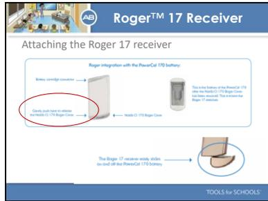
Connecting the Roger 17 receiver to the Naida is easy. Here you can see the PowerCel 170 battery. Take off the 170 Roger Cover by gently pushing on it and then attach the Roger 17 receiver by sliding it on until it clicks into place.
