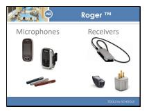
There are two parts to the Roger System. The microphone which is worn by the speaker and the receiver which is worn by the student. The microphone sends the speaker's voice wirelessly, directly to the student's receiver. This provides the student with the ability to hear well despite background noise and distance. Let's look at some of the receiver and microphone options used most commonly in schools.
