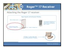
Connecting the Roger 17 receiver to the Naida is easy. Here you can see the PowerCel 170 battery. Take off the 170 Roger Cover by gently pushing on it and then attach the Roger 17 receiver by sliding it on until it clicks into place.
